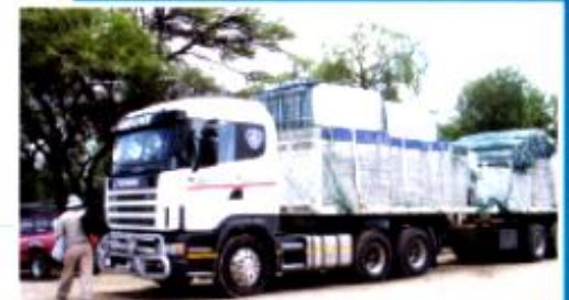
The panels of up to eight houses can be loaded on a single 35t truck.
